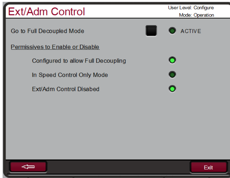
Figure 3-33. Configured for Full Decoupled mode (No Map)
