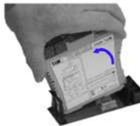
Figure 272: Removing a module from an IOTA
