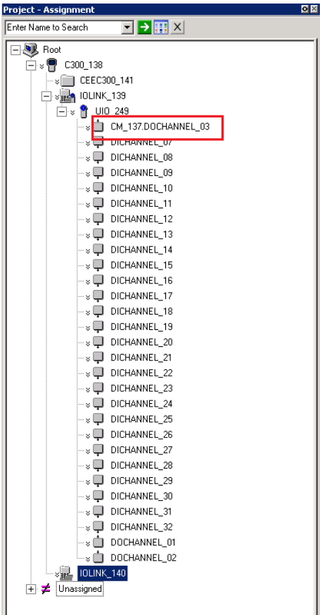
Figure 188: Appearance of DO channels after ganging
