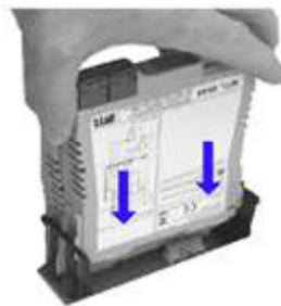
Figure 243: Mounting a module onto an IOTA
