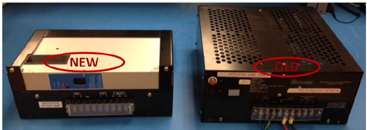
Figure 134: Old and new power supply
