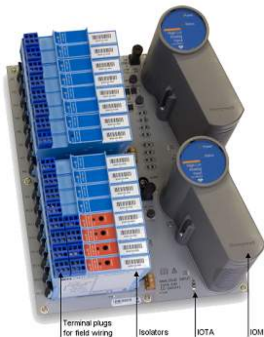
Figure 241: GI/IS board assembly
