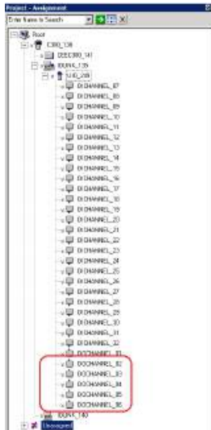
Figure 187: Appearance of DO channels before ganging
