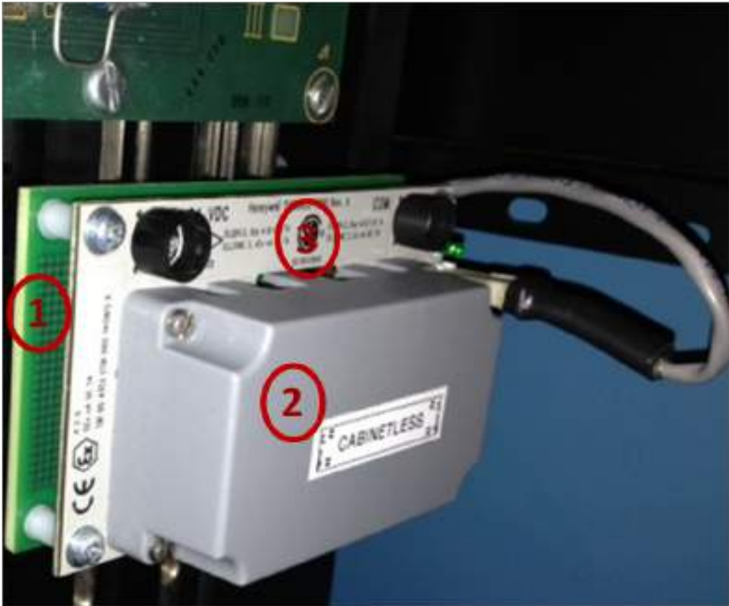
Figure 131: RAM Battery Backup and Battery assembly
