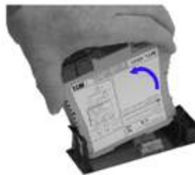
Figure 272: Removing a module from an IOTA
