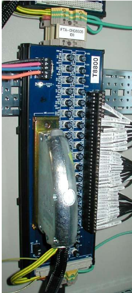
Figure 4-12: Field Termination Assembly
